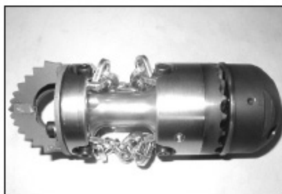
Allstar link-chain-cutter-head to remove incrustation, grease, roots.
